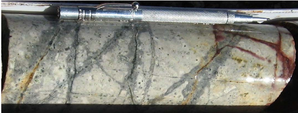
Figure 2: Core from La Tortuga diamond drill hole TOR-DD-001 (at 22m): Porphyry showing strong alteration and stockwork veinlets containing copper sulphide mineralisation (chalcocite and chalcopryite).
